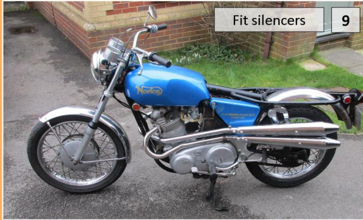
Secure exhaust & heatshields
