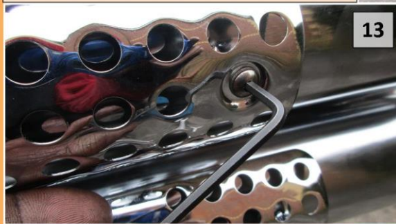
Secure exhaust & heatshields
